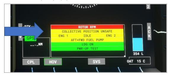
Turn on full pumps: PRIME pumps for start, and FWD and AFT pumps for flight
