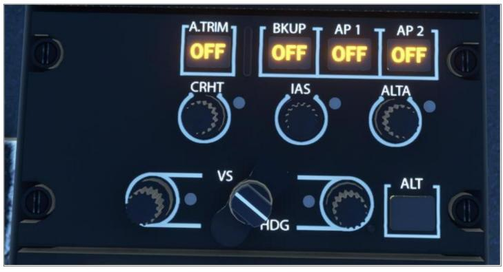
Each amber OFF must be extinguished, by pressing it. When the button is blank, it means the system is ON.
