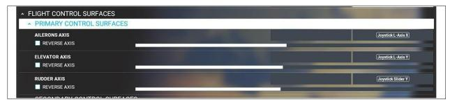
AILERON => controls left & right sideways motion 'cyclic' ELEVATOR => controls forward & backwards motion 'cyclic' RUDDER => controls rotation 'yaw' (right pedal turns clockwise)
